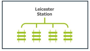
At present, capacity constraints negatively impact Leicester's rail connectivity UK wide. Four tracking the route into the station, (as is the case at Nottingham and Derby stations), will increase reliability, allow for the introduction of enhanced local connections (e.g. to Birmingham, Coventry and the HS2 East Midlands Hub) and future proof Leicester station for further growth.
